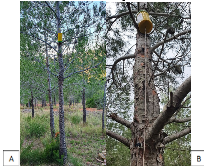
Figure 2. Short-term data-acquisition emplacement in a selected tree. Overview of the installation (A).Close vision of the watertight capsule (B).
